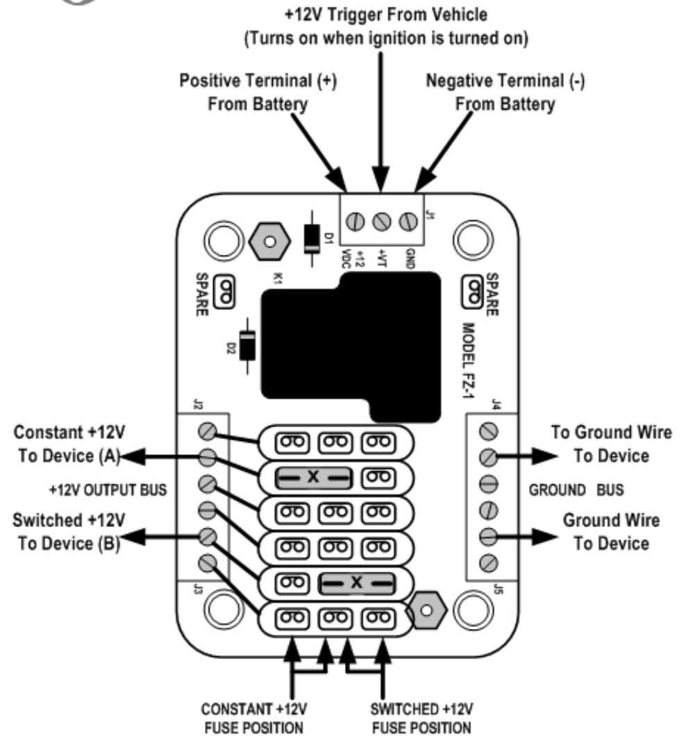
**NOTE:** CHECK YOUR WIRING BEFORE APPLYING POWER TO THE FZ-1 OR TO ANY DEVICES.
